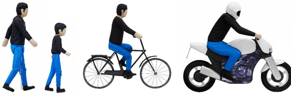
Figure 5-1: Euro NCAP VRU Targets (EPTa, EPTc, EBT and EMT)
